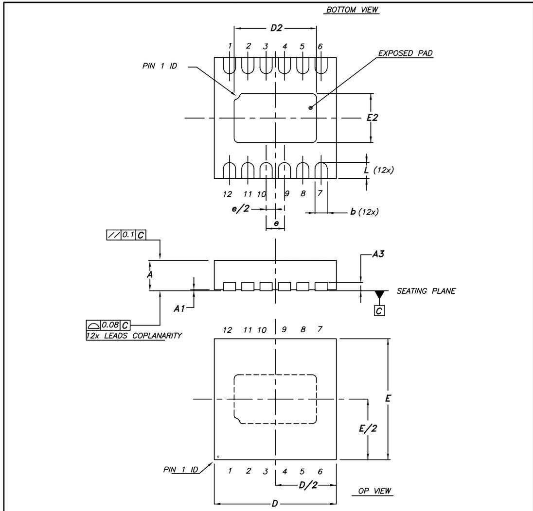
Table 9: DFN12L (3x3x0.75 mm) package mechanical data
