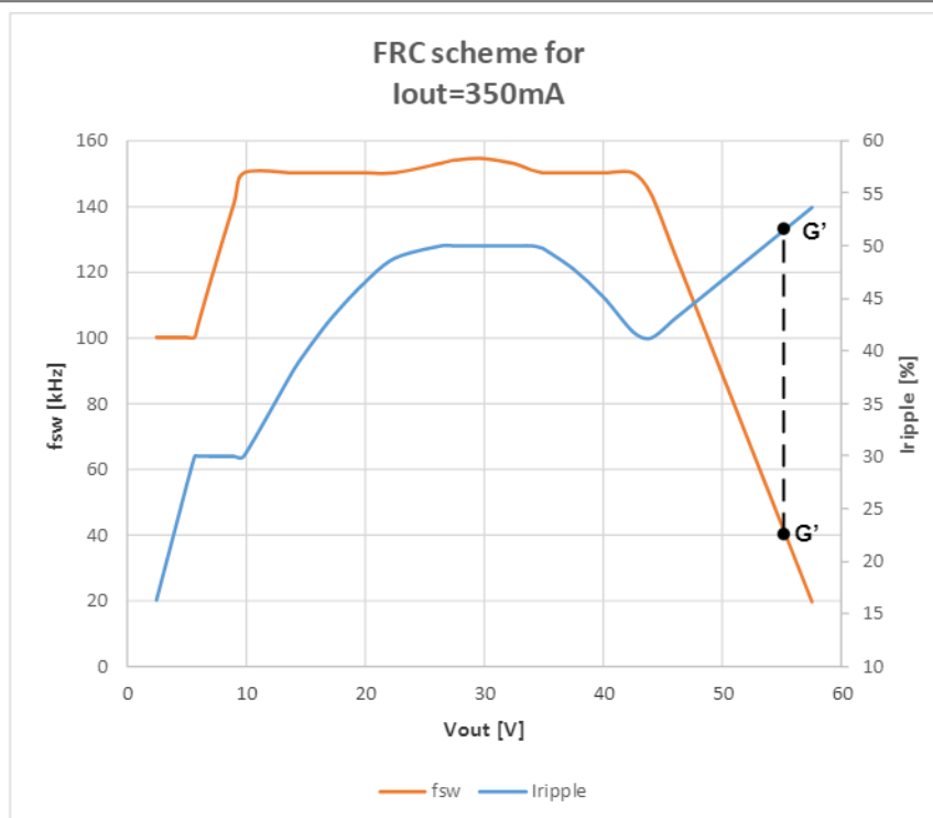
Figure 21. Operating Point determined by Toff_min criteria
