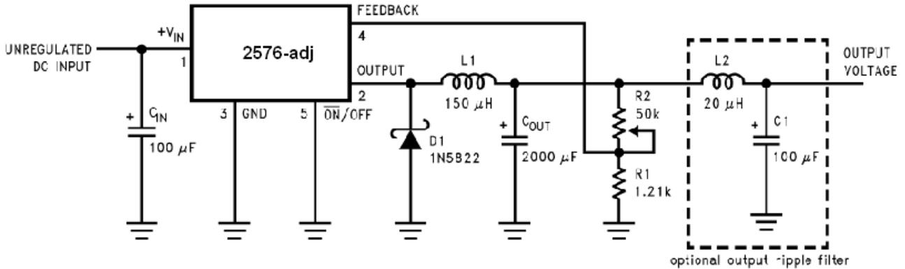
**FIGURE 10. Adjustable 1A Power Supply with Low Output Ripple**
