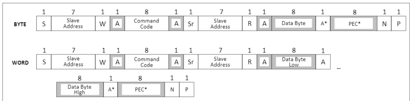
Figure 59: SMBus Read Byte/Word
