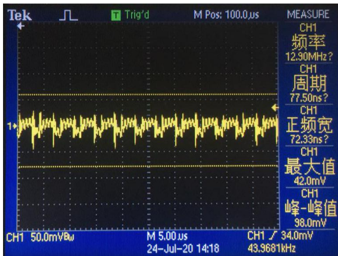
Noise ( V_{IN} = 48V , I_O = 0.5A , 5 ~ 20MHz bandwidth)
