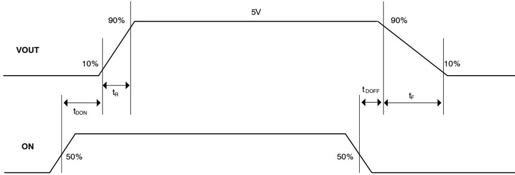
Figure 4. Normal ON/OFF Operation by ON (POL = GND)
