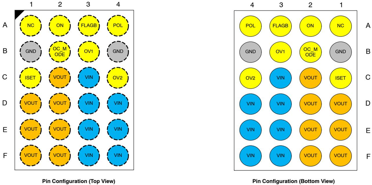
**Figure 3. Pin Configuration**
