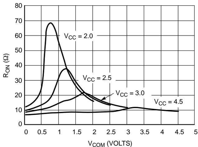
Figure 8.  $R_{ON}$  vs.  $V_{COM}$  and  $V_{CC}$  (@25°C)
