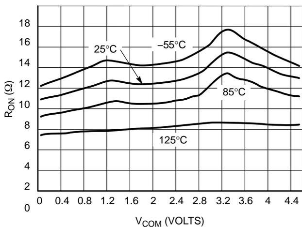
Figure 12.  $R_{ON}$  vs.  $V_{COM}$  and Temperature,  $V_{CC} = 4.5$  V
