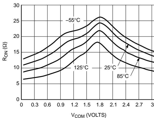
Figure 11.  $R_{ON}$  vs.  $V_{COM}$  and Temperature,  $V_{CC} = 3.0$  V
