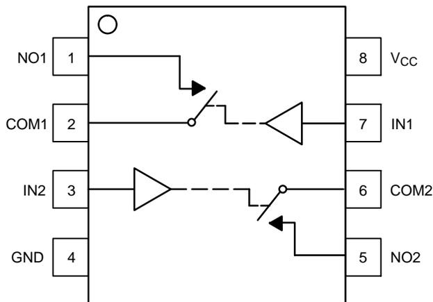
Figure 1. Pinout
