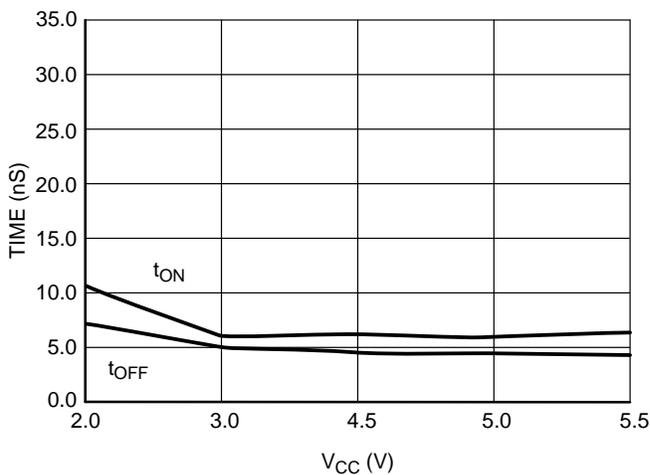
Figure 13. Switching Time vs. Supply Voltage,  $T = 25^\circ\text{C}$
