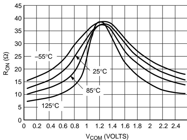
Figure 10.  $R_{ON}$  vs.  $V_{COM}$  and Temperature,  $V_{CC} = 2.5$  V
