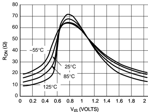
Figure 9.  $R_{ON}$  vs.  $V_{COM}$  and Temperature,  $V_{CC} = 2.0$  V
