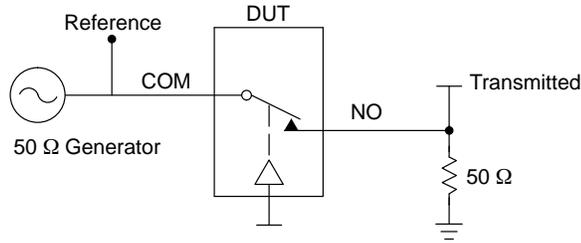
Channel switch control/s test socket is normalized. Off isolation is measured across an off channel. On loss is the bandwidth of an On switch.  $V_{ISO}$ , Bandwidth and  $V_{ONL}$  are independent of the input signal direction.
