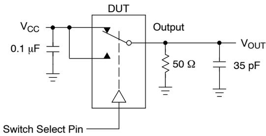
Figure 4.  $t_{BMM}$  (Time Break-Before-Make)
