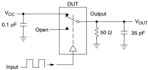
Figure 5.  $t_{ON}/t_{OFF}$
