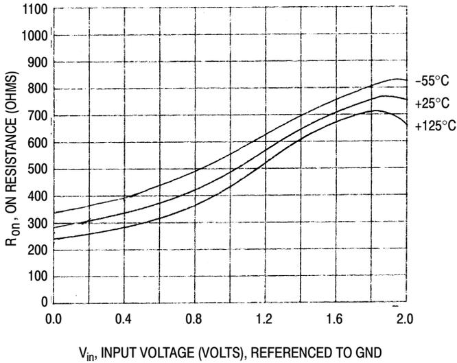
Figure 6. Typical On Resistance  $V_{CC} = 2V$
