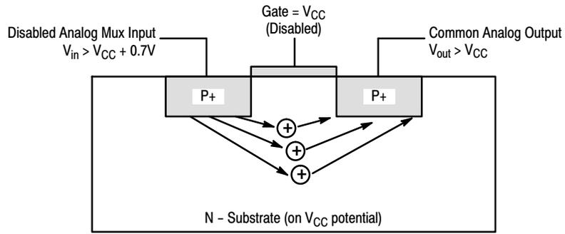
**Figure 24. Diagram of Bipolar Coupling Mechanism**
