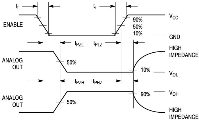
**Figure 21. Propagation Delays, Enable to Analog Out**
