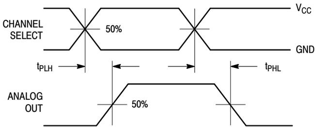
Figure 17. Propagation Delays, Channel Select to Analog Out
