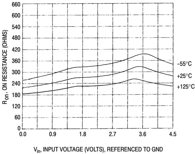
Figure 8. Typical On Resistance  $V_{CC} = 4.5V$
