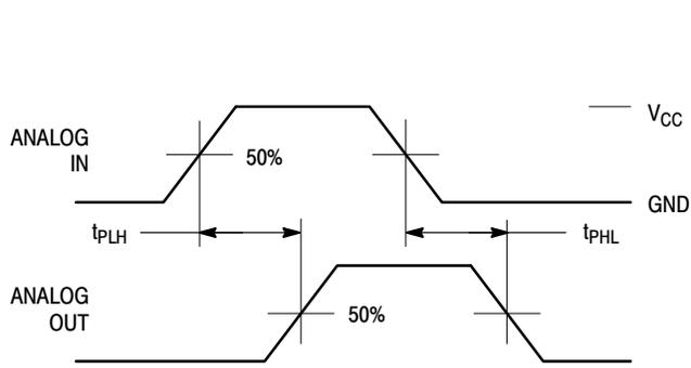
**Figure 19. Propagation Delays, Analog In to Analog Out**
