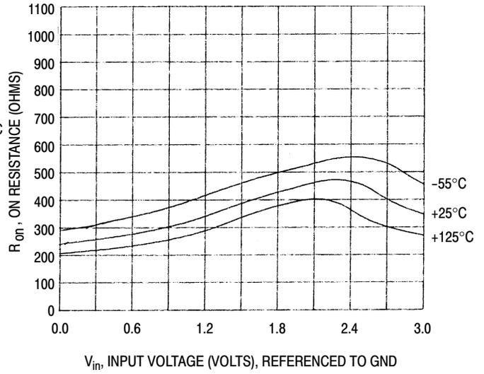
Figure 7. Typical On Resistance  $V_{CC} = 3V$
