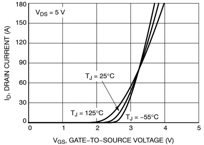
Figure 2. Transfer Characteristics
