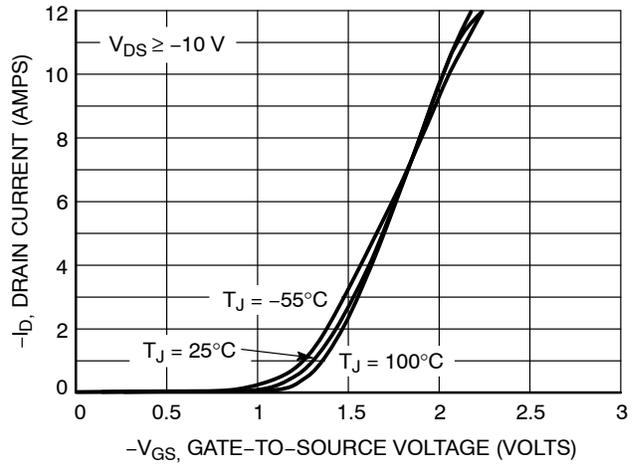
Figure 2. Transfer Characteristics
