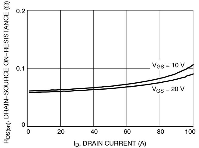
**Figure 4. On-Resistance Variation vs. Drain
