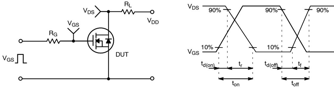
Figure 20. Resistive Switching Test Circuit & Waveforms
