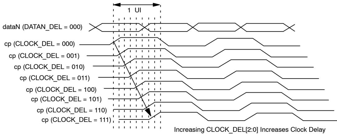
**Figure 12. Delaying the Clock with Respect to Data**
