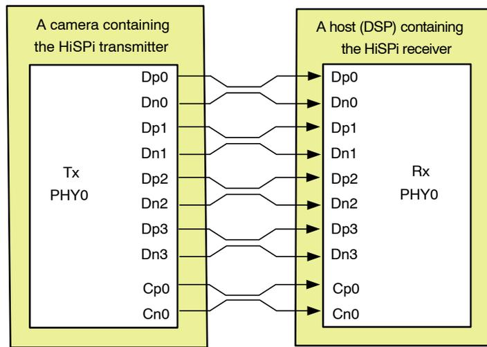
**Figure 9. HiSPi Transmitter and Receiver Interface Block Diagram**
