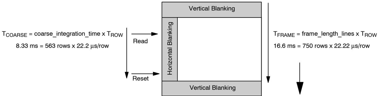
Figure 15. Example of 8.33 ms Integration in 16.6 ms Frame
