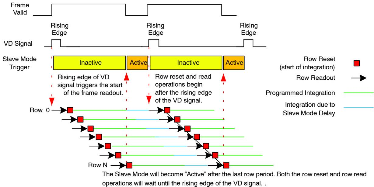
Note: The integration of the last row is started before the end of the programmed integration for the first row.
