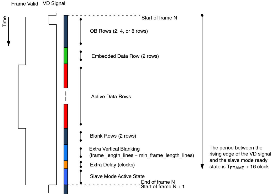
**Figure 26. Slave Mode Active State and Vertical Blanking**
