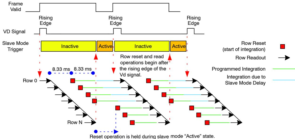
Note: The sensor read pointer will have paused at row 0 while the shutter pointer pauses at row N/2. The extra integration caused by the slave mode delay will only be seen by rows 0 to N/2. The example below is for a frame readout period of 16.6 ms while the integration time is configured to 8.33 ms.
