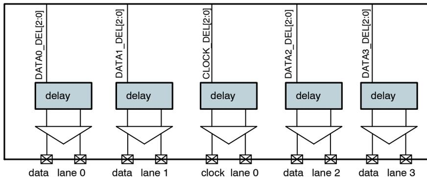
**Figure 11. Block Diagram of DLL Timing Adjustments**
