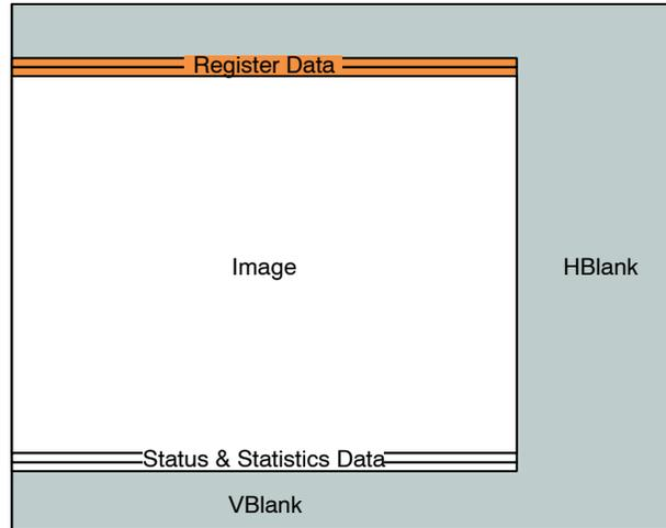
**Figure 32. Frame Format with Embedded Data Lines Enabled**
