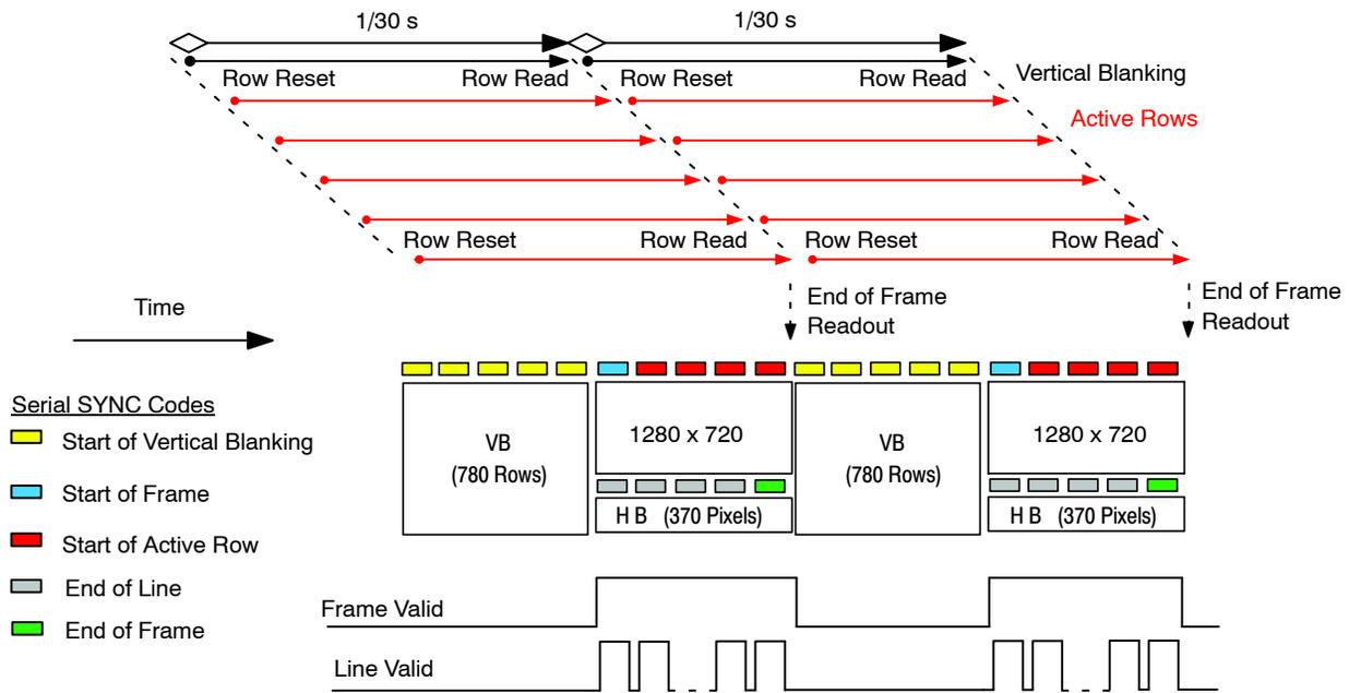
Note: The frame valid and line valid signals mentioned in this diagram represent internal signals within the sensor. The SYNC codes represented in this diagram represent the HiSPi Streaming-SP protocol.
