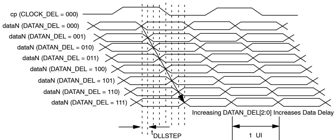
**Figure 13. Delaying Data with Respect to the Clock**
