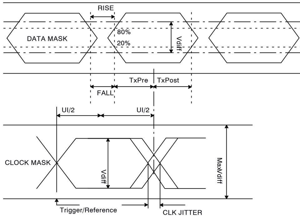
**Figure 47. Eye Diagram for Clock and Data Signals**
