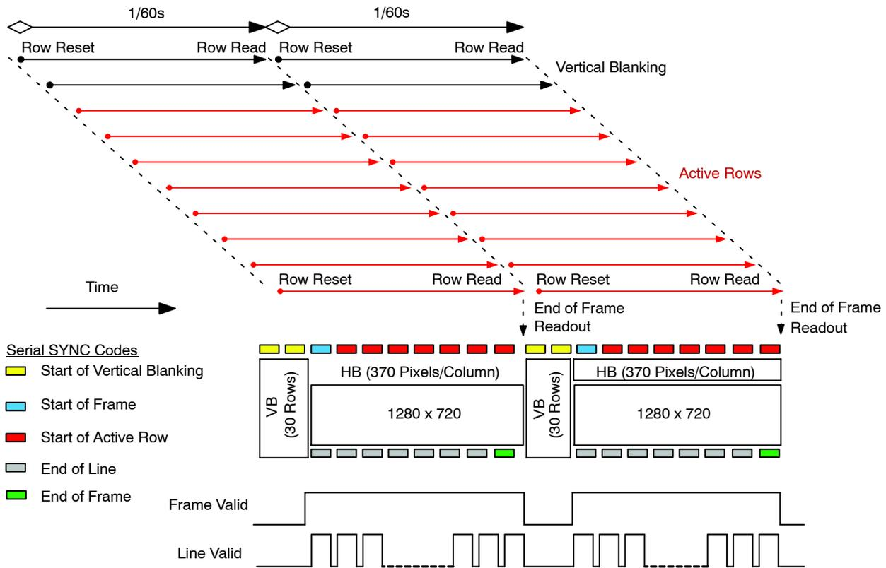
Note: The frame valid and line valid signals mentioned in this diagram represent internal signals within the sensor. The SYNC codes represented in this diagram represent the HiSPi Streaming-SP protocol.
