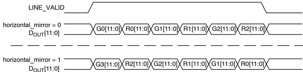
**Figure 21. Effect of Horizontal Mirror on Readout Order**
