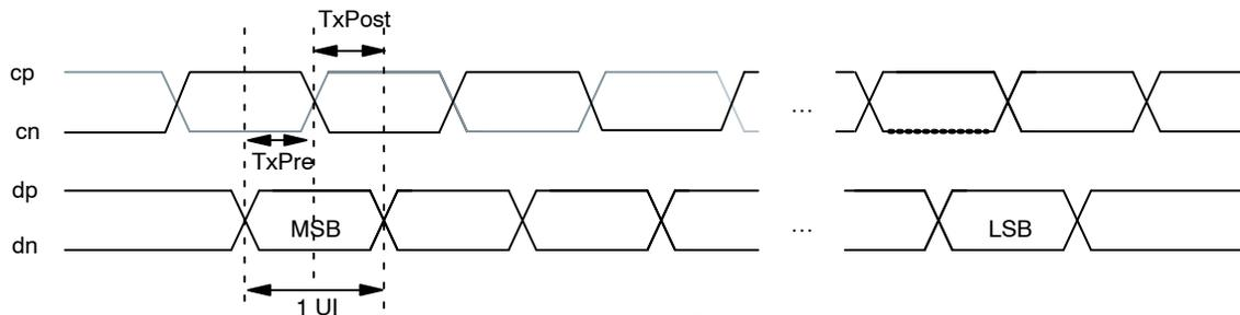
**Figure 10. Timing Diagram**
