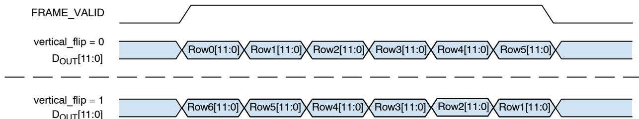
**Figure 22. Effect of Vertical Flip on Readout Order**
