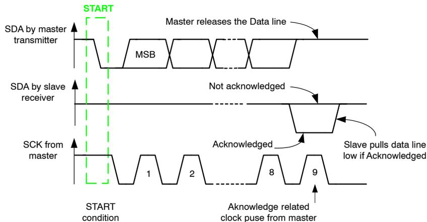
**Figure 26. Acknowledge on the I<sup>2</sup>C-bus**
