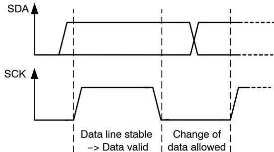
Figure 23. Bit Transfer on the I<sup>2</sup>C-bus
