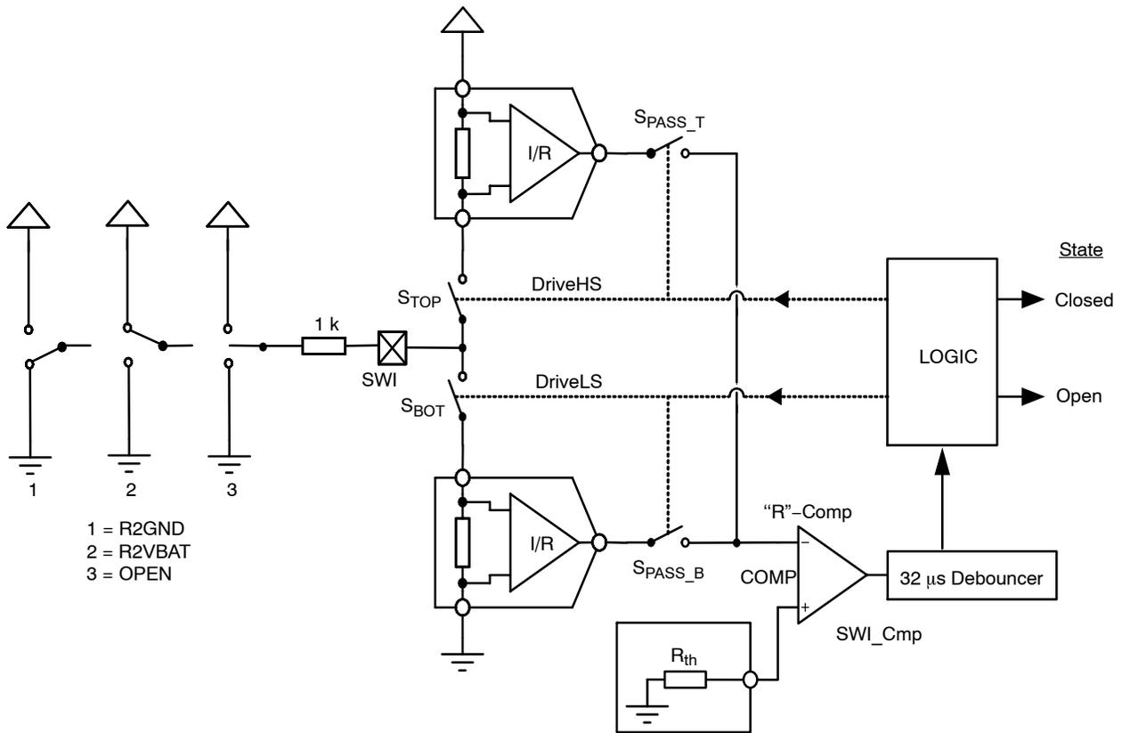
Figure 12. Simplified Schematic Diagram of the SWI Comparator
