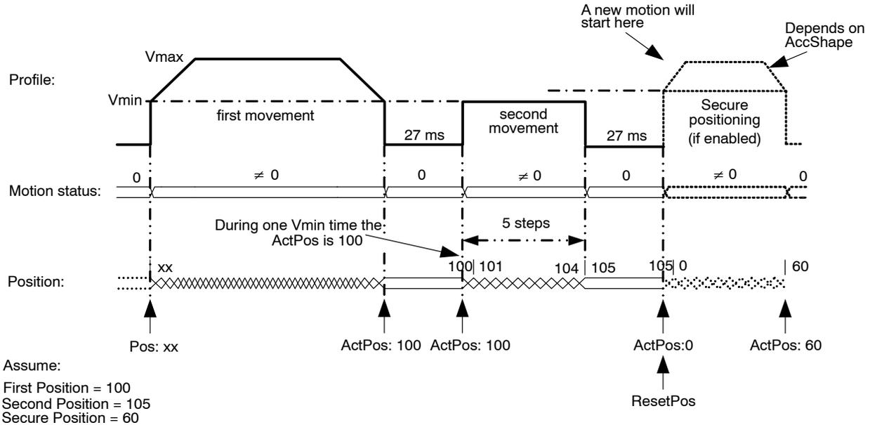
**Figure 8. Dual Positioning**
