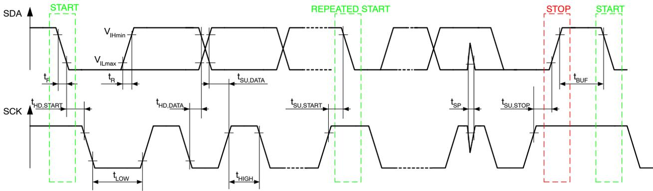
Figure 5. I<sup>2</sup>C Timing Diagrams
