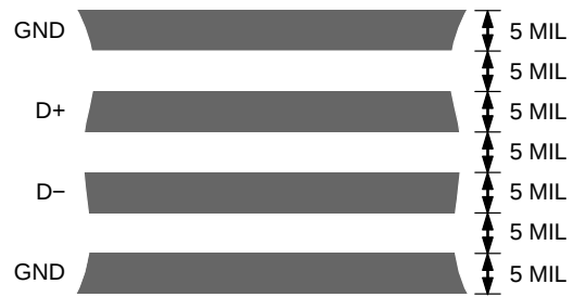
Figure 22. Typical Arrangement of Signal Tracks
