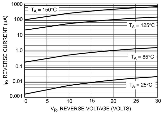
Figure 3. Leakage Current
