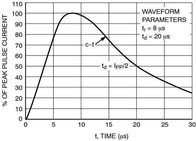
Figure 1. Pulse Waveform,  $8 \times 20 \mu\text{s}$
