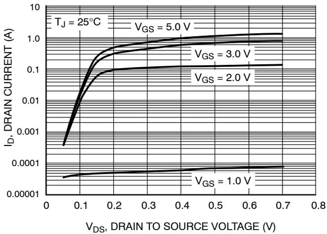
Figure 2. Output Characteristics
