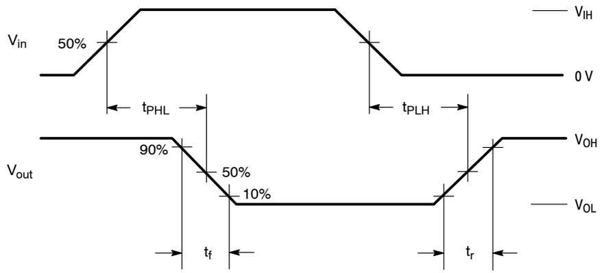
Figure 1. Switching Waveforms
