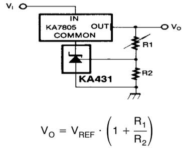
Figure 13. Output Control for Three-Terminal Fixed Regulator
