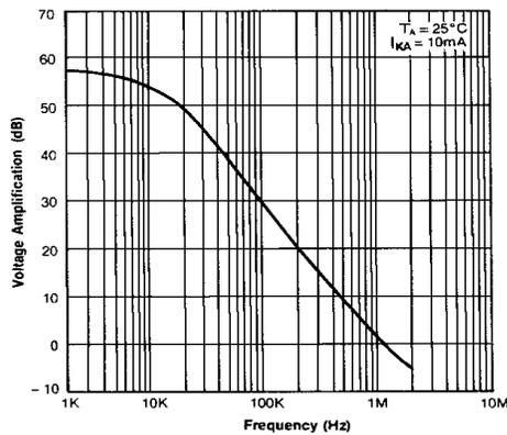
Figure 9. Small Signal Voltage Amplification vs. Frequency
