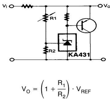
Figure 14. High-Current Shunt Regulator
