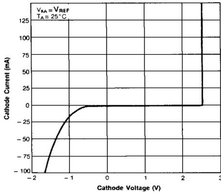
Figure 5. Cathode Current vs. Cathode Voltage
