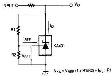
Figure 3. Test Circuit for  $V_{KA} \geq V_{REF}$
