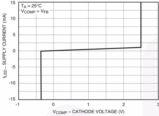
Fig. 9b – LED Current vs. Cathode Voltage
