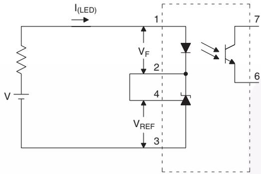
Figure 1.  $V_{REF}$ ,  $V_F$ ,  $I_{LED}$  (min.) Test Circuit
