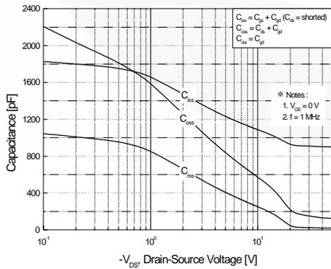
**Figure 5. Capacitance Characteristics**
