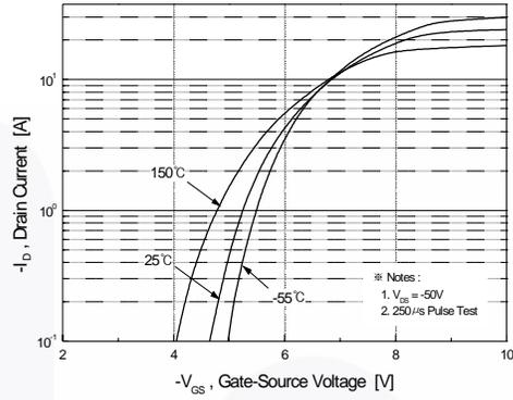
**Figure 2. Transfer Characteristics**
