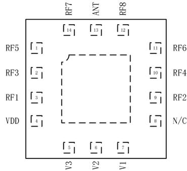
**Figure 2. FM3418C Pinout - 14-Pin QFN (Top View)**
