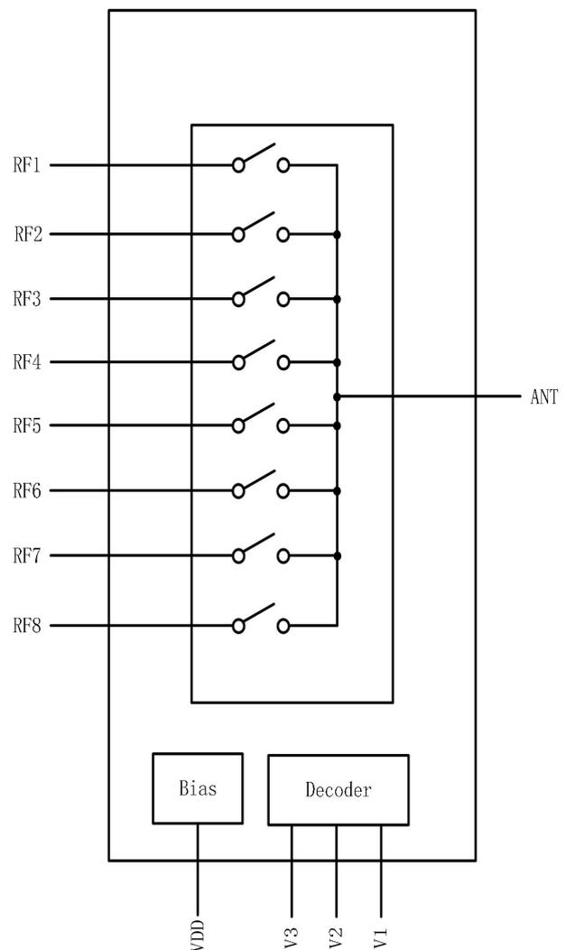
**Figure 1. FM3418C Block Diagram**
