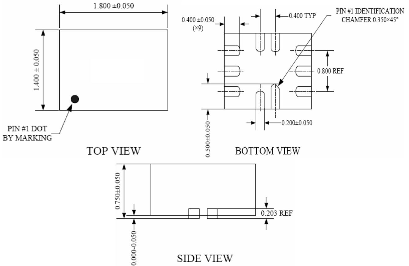
**Note: All linear dimensions are in millimeters.**
