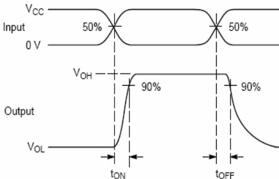
Figure 2.  $t_{ON} / t_{OFF}$
