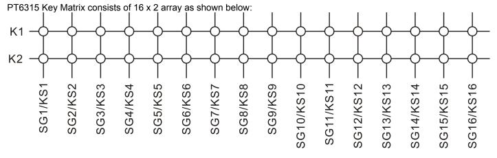
Each data inputted by each key are stored as follows. They are read by a READ Command, starting from the last significant bit. When the most significant bit of the data (SG16, b7) has been read, the least significant bit of the next data (SG1, b0) is read.
