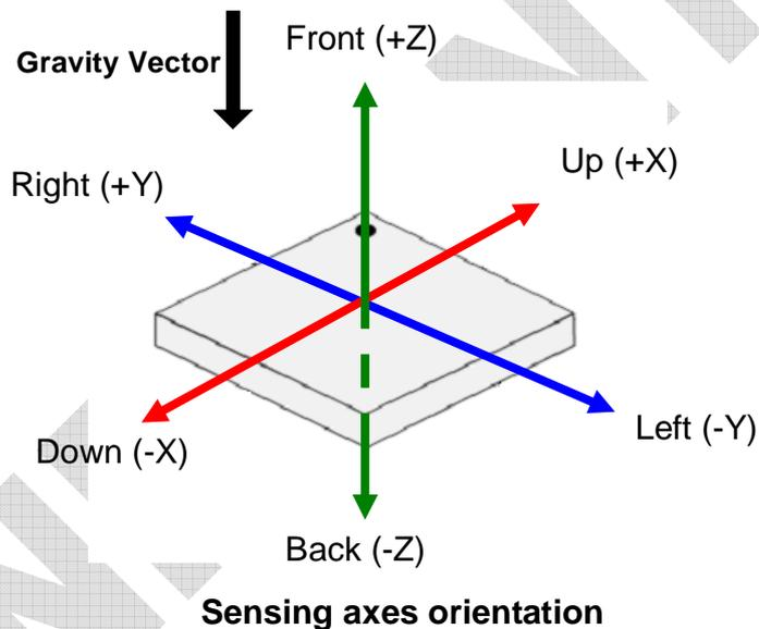
The following table lists all corresponding output signals on X, Y, and Z while the sensor is at rest or at uniform motion in a gravity field under assumption of a  $\pm 2g$  range setting, a 12 bit resolution, and a top down gravity vector as shown above.
