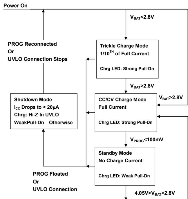
Figure1. State Diagram of a Typical Charge Cycle
