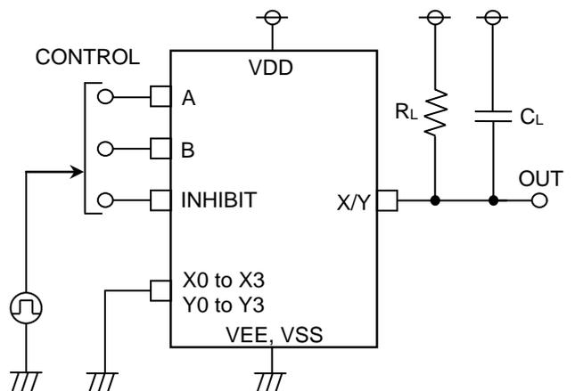
Figure 6. Test Circuit 3 ( $t_{PZL}, t_{PLZ}$ )
