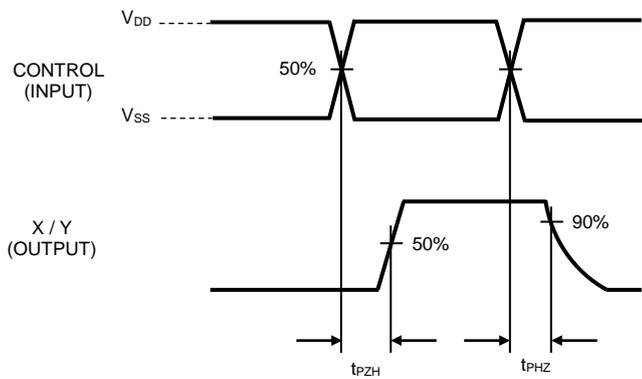
Figure 3. Propagation Delay Time (CONTROL (A,B,INHIBIT)→OUT) ( $t_{PLH}, t_{PHL}$ )
