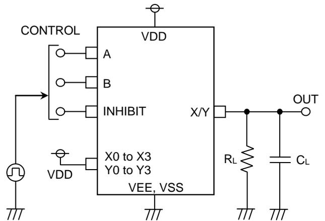
Figure 4. Test Circuit 2 ( $t_{PZH}, t_{PHZ}$ )
