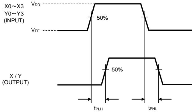
Figure 1. Propagation Delay Time (IN→OUT) ( $t_{PLH}, t_{PHL}$ )
