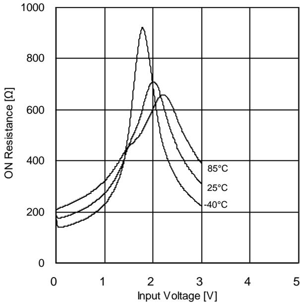
Figure 7. ON Resistance vs Input Voltage
