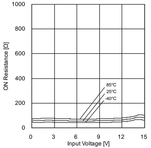
Figure 10. ON Resistance vs Input Voltage
