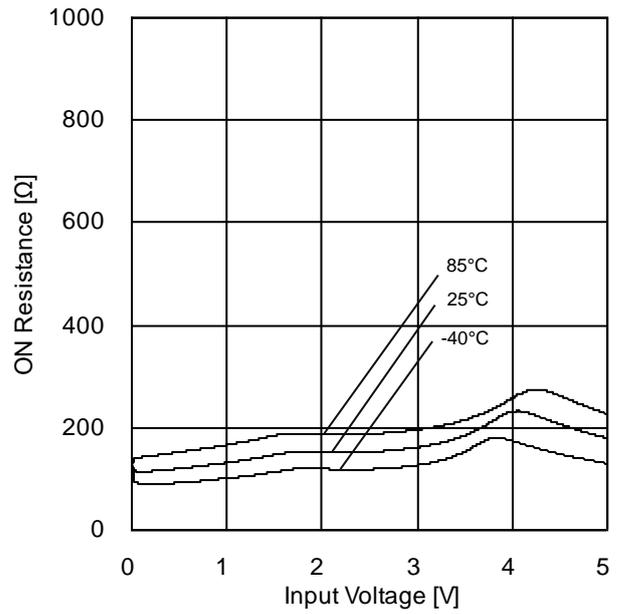
Figure 8. ON Resistance vs Input Voltage
