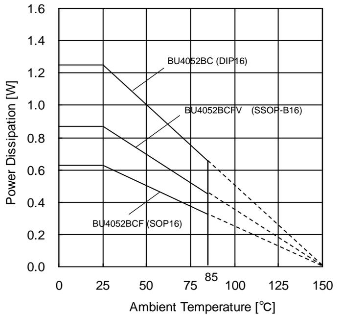
Figure 22. Derating Curve
