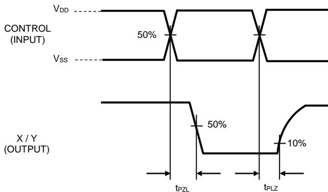
Figure 5. Propagation Delay Time (CONTROL (A,B,INHIBIT)→OUT) ( $t_{PZL}, t_{PLZ}$ )
