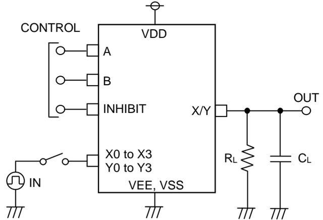
Figure 2. Test Circuit 1 ( $t_{PLH}, t_{PHL}$ )
