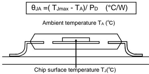
Figure 21. Thermal Resistance
