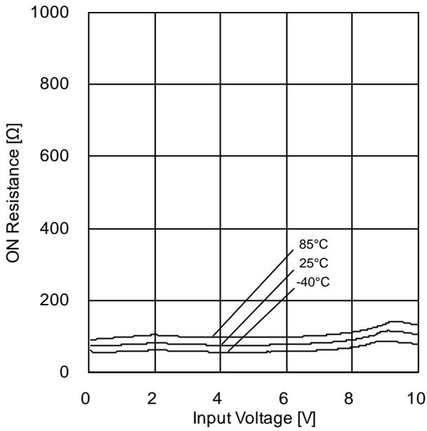
Figure 9. ON Resistance vs Input Voltage
