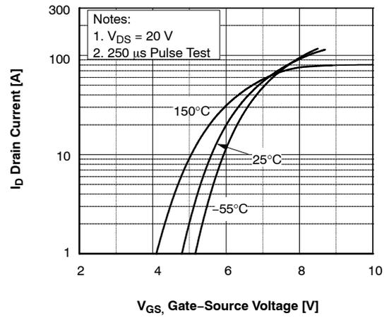
Figure 2. Transfer Characteristics
