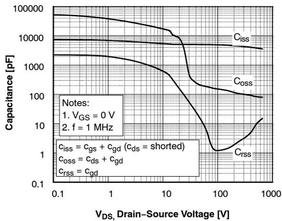
Figure 5. Capacitance Characteristics
