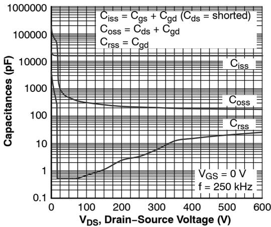
Figure 5. Capacitance Characteristics
