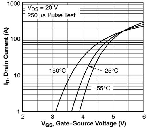
Figure 2. Transfer Characteristics
