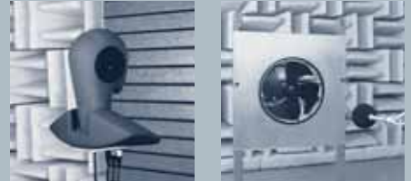
Room for precision noise measuring
