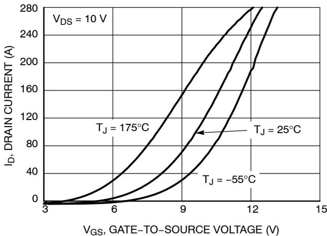
Figure 5. Transfer Characteristics
