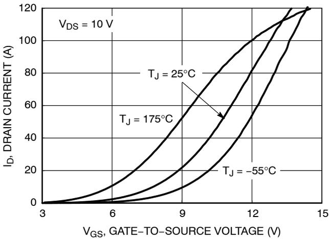
Figure 5. Transfer Characteristics
