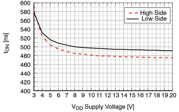
**Figure 29. Turn-On Propagation Delay vs.  $V_{DD}$  Supply Voltage**
