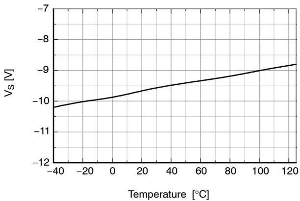
Figure 26. Allowable Negative V<sub>S</sub> vs. Temperature
