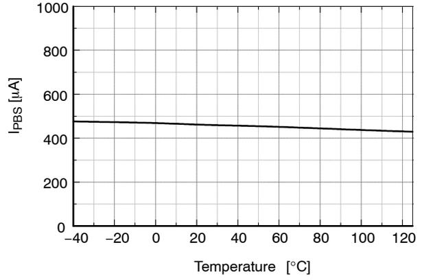
Figure 17. Operating V<sub>BS</sub> Supply Current vs. Temperature
