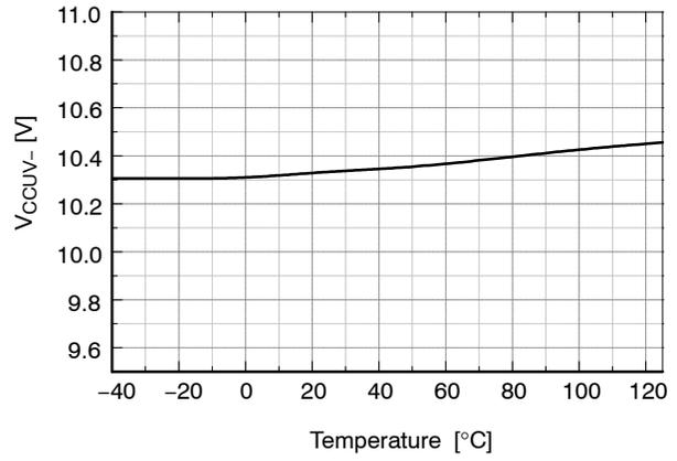
Figure 19. V<sub>CC</sub> UVLO- vs. Temperature
