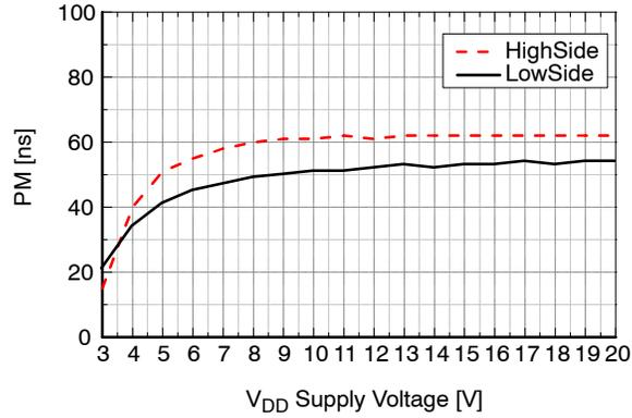
Figure 34. Output Pulse-Width Matching vs. V<sub>DD</sub> Supply Voltage
