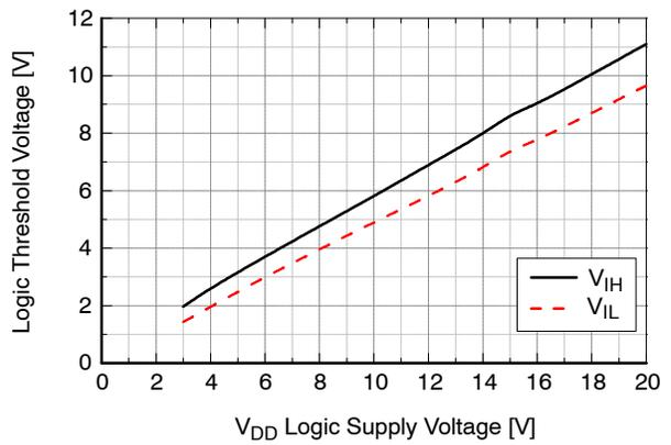
Figure 27. Input Logic (HIN&LIN) Threshold vs. V<sub>DD</sub> Supply Voltage
