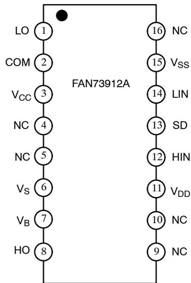
**Figure 3. Pin Connections – Wide 16-SOIC
