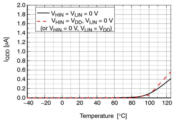
Figure 13. Quiescent V<sub>DD</sub> Supply Current vs. Temperature
