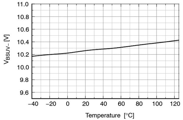
Figure 21. V<sub>BS</sub> UVLO- vs. Temperature
