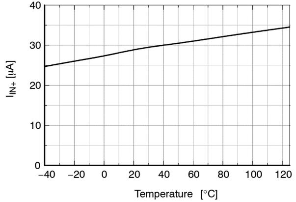
Figure 11. Logic Input High Bias Current vs. Temperature
