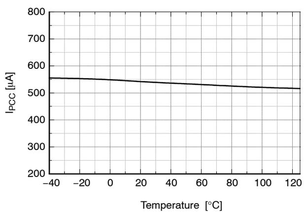
Figure 15. Operating V<sub>CC</sub> Supply Current
