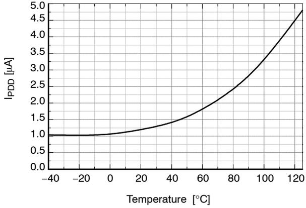
Figure 16. Operating V<sub>DD</sub> Supply Current
