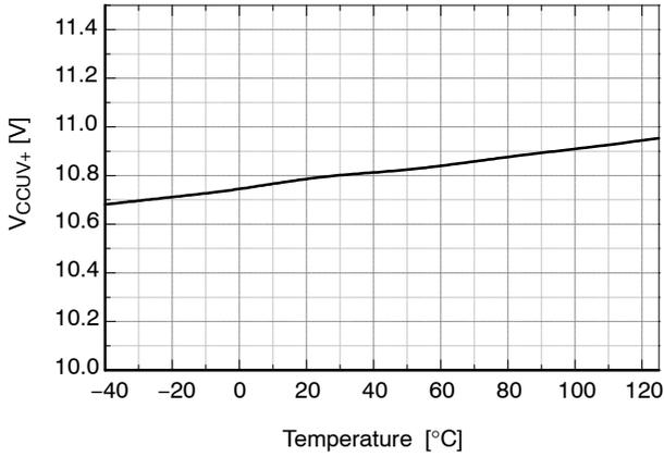
Figure 18. V<sub>CC</sub> UVLO+ vs. Temperature
