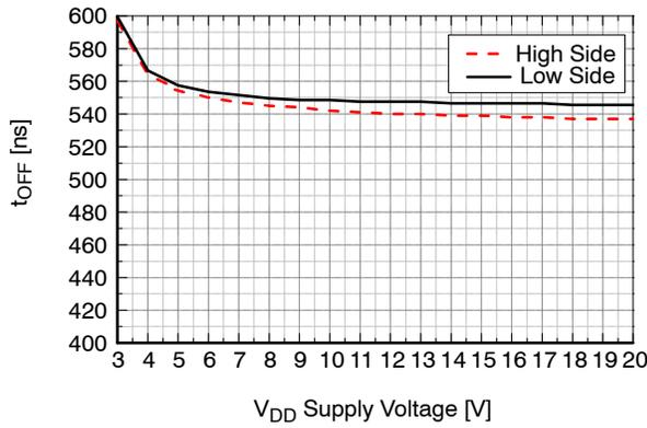
**Figure 30. Turn-Off Propagation Delay vs.  $V_{DD}$  Supply Voltage**
