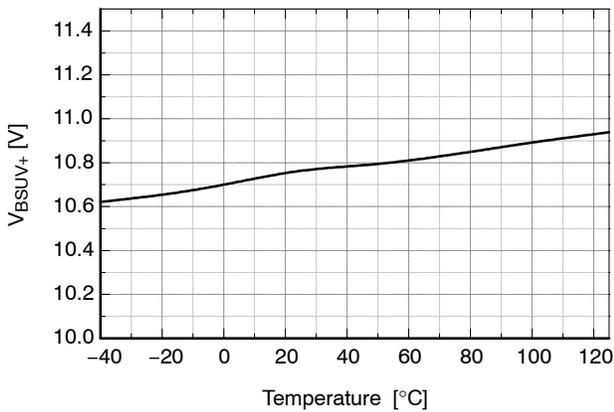
Figure 20. V<sub>BS</sub> UVLO+ vs. Temperature
