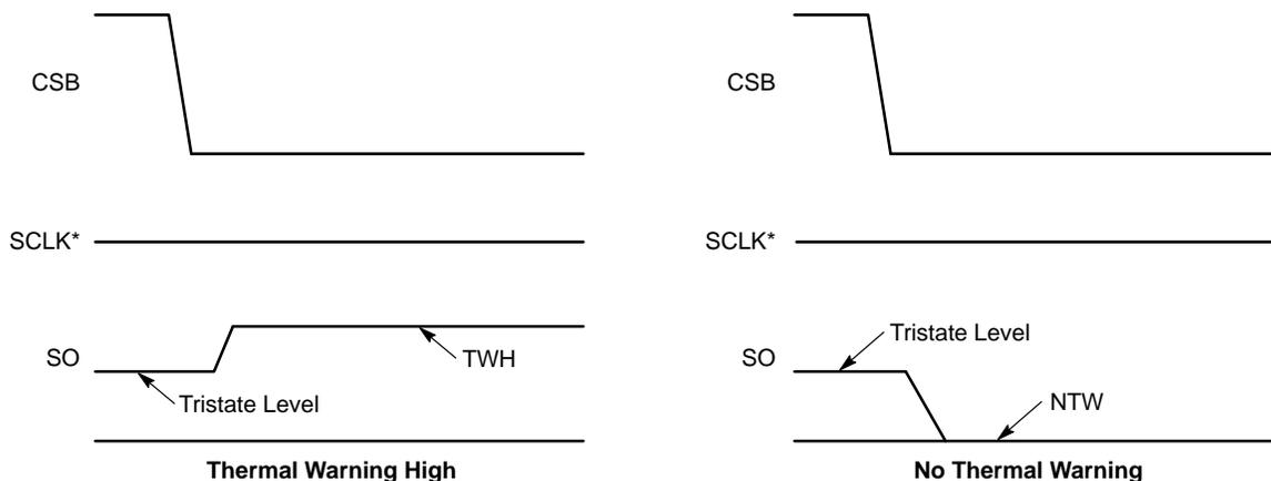
\*SCLK can be high or low in order to maintain the thermal information on SO. Toggling SCLK will cause other output bits to shift out.
