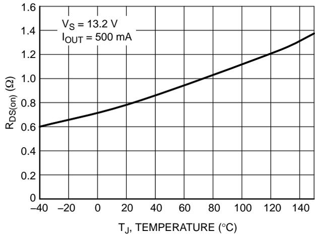
Figure 6. (Source / Sink)  $R_{DS(on)}$  vs. Temperature
