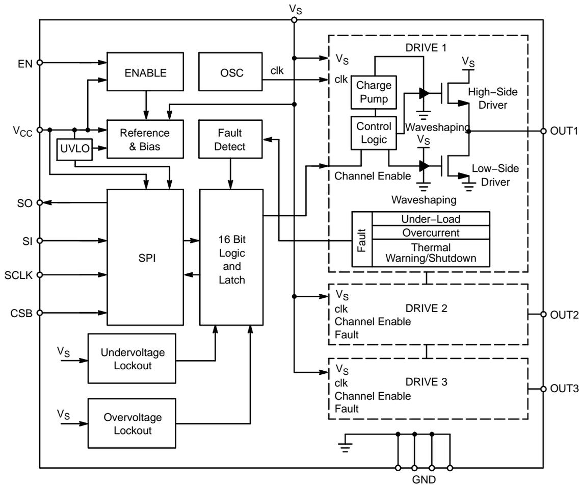
Figure 2. Block Diagram
