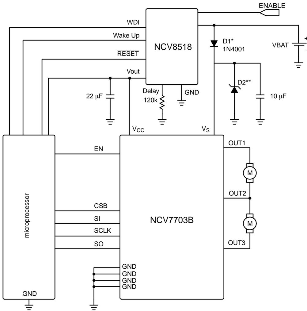
\* D1 optional. For use where reverse battery protection is required.
