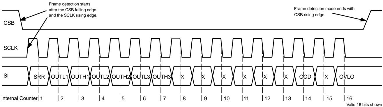
Figure 12. Frame Detection
