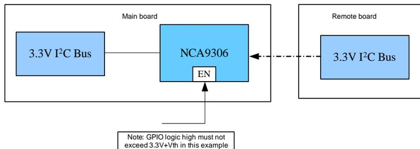
Figure 6.4 An example of connecting a remote board to a main board (backplane)
