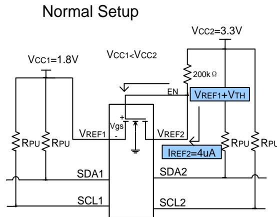
Figure 6.1 Normal Setup
