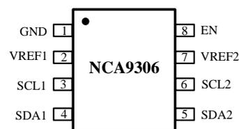
Figure 1. NCA9306 Block Diagram
