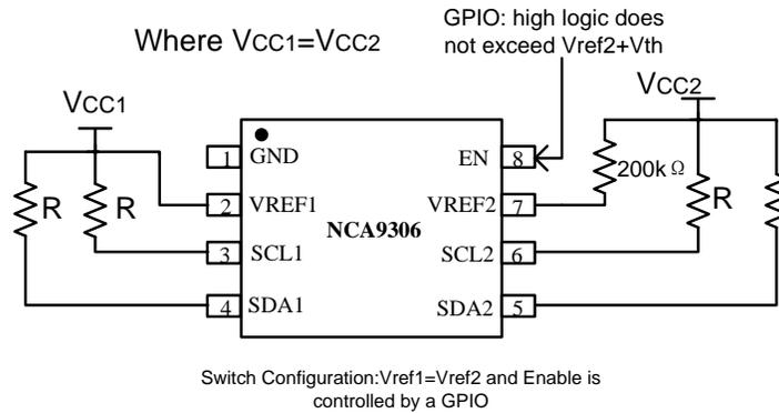
Figure 6.5 Switch Configuration
