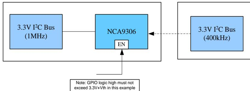
Figure 6.3 Example of an I<sup>2</sup>C bus with multiple supported frequencies
