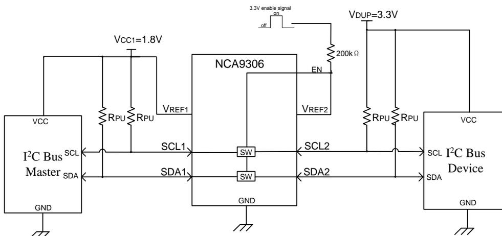
Figure 7.2 Typical Application Circuit (Switch Enable Control)
