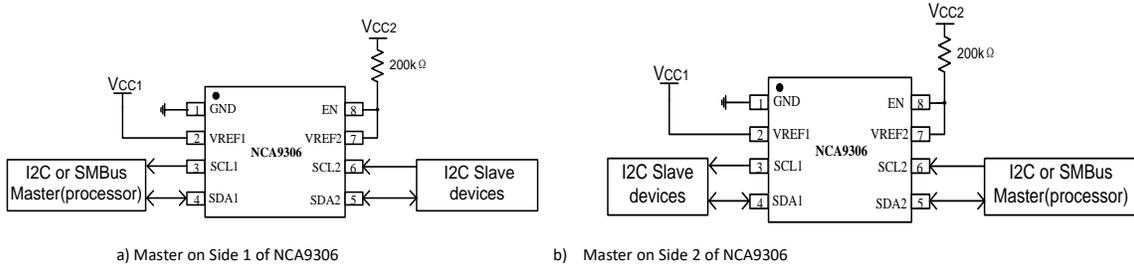
Figure 6.7 Master on Side 1 or Side 2 of NCA9306
