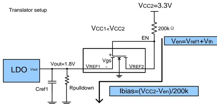
Figure 6.9 Example with Leakage current path when using an LDO
