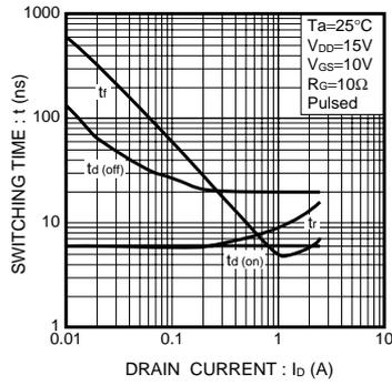
Fig.2 Switching Characteristics
