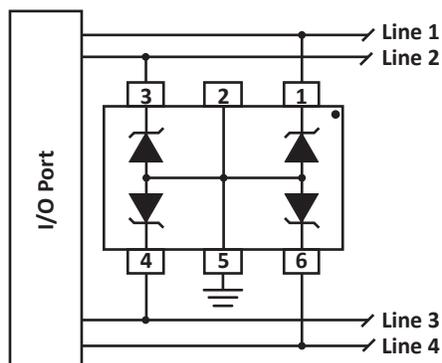
**FIGURE 1 - COMMON-MODE I/O PORT PROTECTION (UNIDIRECTIONAL)**
