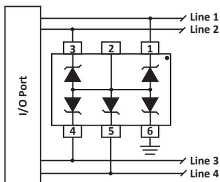
**FIGURE 1 - COMMON-MODE I/O PORT PROTECTION (BIDIRECTIONAL)**
