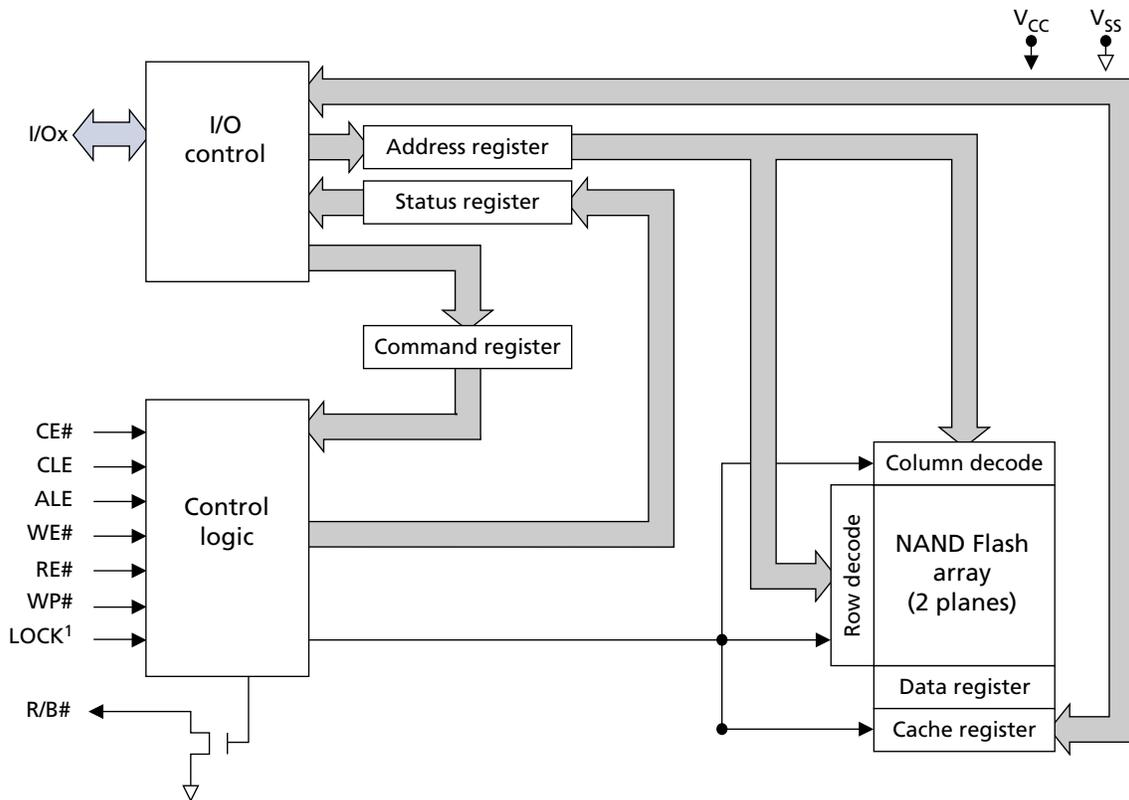
Note: 1. The LOCK pin is used on the 1.8V device.
