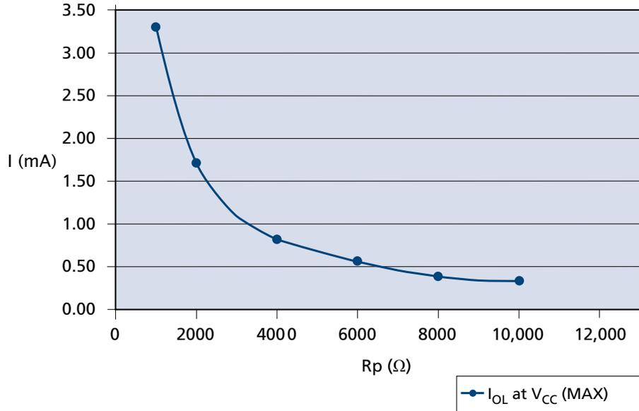
Figure 21:  $I_{OL}$  vs.  $R_p$  (1.8V  $V_{CC}$ )
