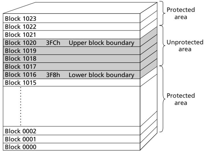
Figure 53: Flash Array Protected: Invert Area Bit = 1
