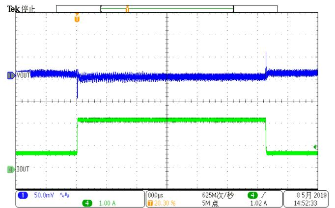
Figure 14. Load Transient
