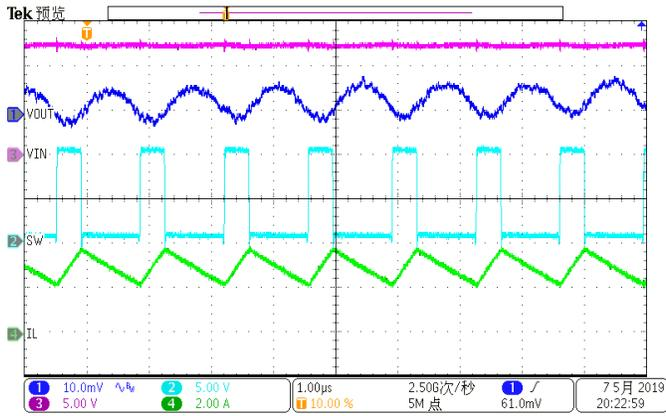
Figure 9. SW node waveform and Output Ripple
