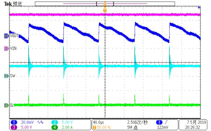
Figure 10. SW node Waveform and Output Ripple
