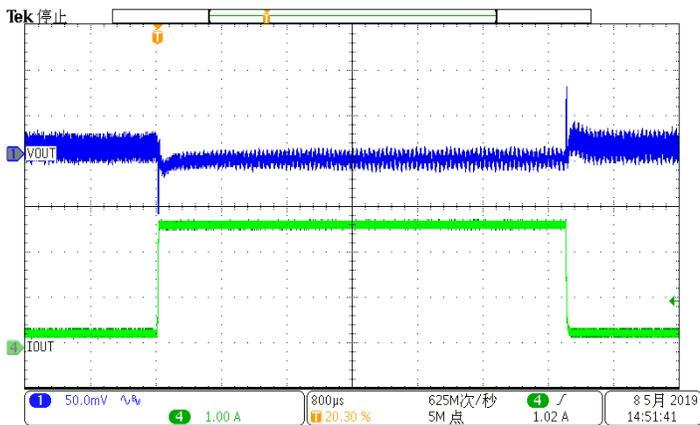
Figure 13. Load Transient
