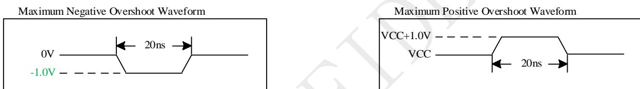
Figure 5-1 Maximum Overshoot Waveform
