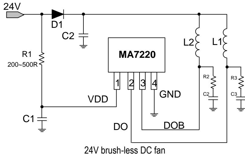
**Note1:** C2(Optional) is for power stabilization, Recommended E-Cap 2.2uF/50V and D1 (Optional) is a reverse protect diode.
