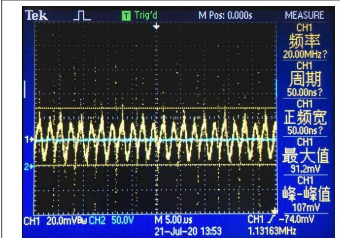
Noise (VIN = 57V, IO = 1.25A, 5 ~ 20MHz bandwidth)
