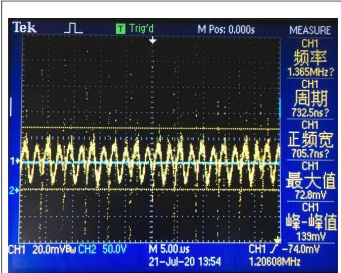
Noise (VIN = 42V, IO = 1.25A, 5 ~ 20MHz bandwidth)
