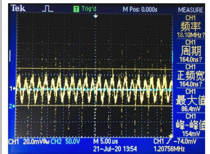
Noise (VIN = 48V, IO = 1.25A, 5 ~ 20MHz bandwidth)
