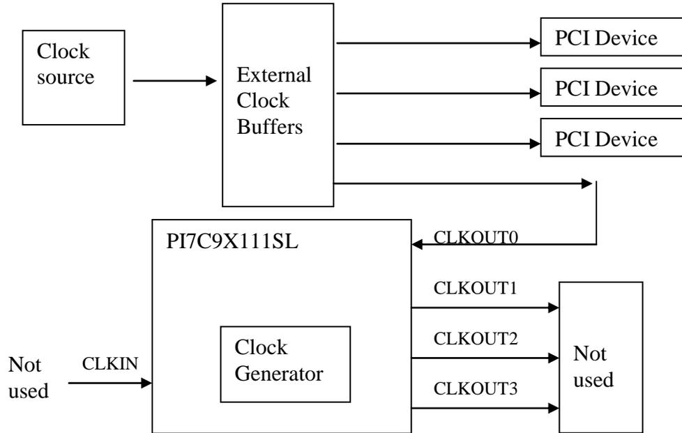
In this configuration, user simply connects the external clock from the clock buffers to CLKOUT0. And user needs to make sure the clock is preset (toggling) before the fundamental reset de-asserted (e.g. PERST\_L when forward mode, and RESET\_L when reverse mode).
