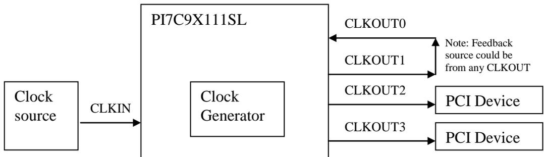
In this configuration, user simply connects the external clock source to CLKIN pin. And user needs to make sure the clock is preset (toggling) before the fundamental reset de-asserted (e.g. PERST\_L when forward mode, and RESET\_L when reverse mode). In this mode, the frequency is the same as the input clock source.
