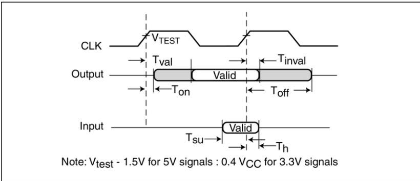
Table 16-4 specifies the voltage and timing requirements for the input clock signals.
