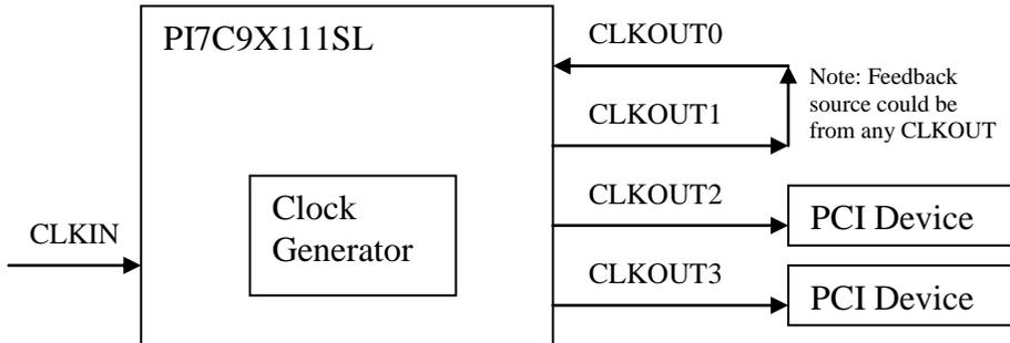
Topology of external clock source and internal clock buffering:
