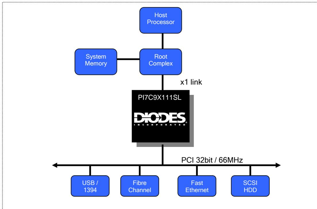
In reverse mode (REVRSB=1), PI7C9X111SL becomes a PCI-to-PCI Express bridge that its PCI bus interface is connected to the PCI Host Chipset between and the PCI Express x1 link. It enables the legacy PCI Host Systems to provide PCI Express Interface capability.
