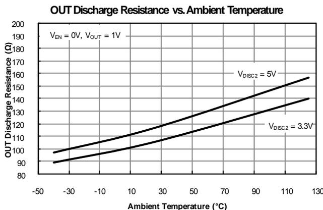
**Performance Characteristics** (@  $T_A = +25^\circ\text{C}$ ,  $V_{IN} = 5\text{V}$ ,  $C_{IN} = C_{OUT} = 10\mu\text{F}$ ,  $V_{EN} = 3.3\text{V}$ ,  $V_{FRS} = 0\text{V}$ ,  $C_{DV}/DT = 1\text{nF}$ ,  $R_{LIM} = 54.9\text{k}\Omega$ ,  $R_{LIM} = 27\text{k}\Omega$ , unless otherwise specified.) (continued)
