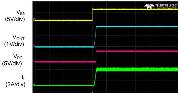
**Enable Turn off Characteristic (I<sub>OUT</sub>=3A)**
