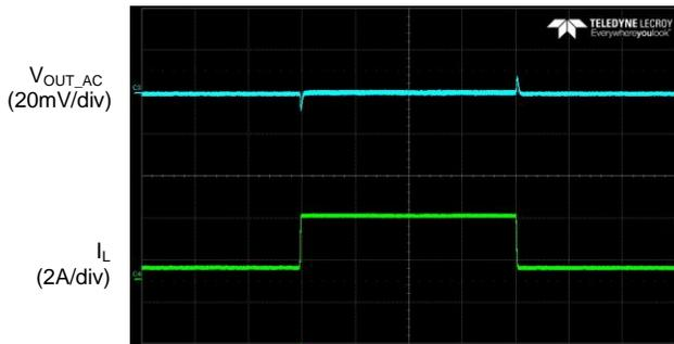
**Load Transient (I<sub>OUT</sub>=2A to 3A)**
