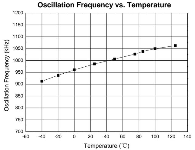
**Typical Performance Characteristics** (@T<sub>A</sub> = +25°C, V<sub>IN</sub> = 5V, V<sub>OUT</sub> = 1.8V, unless otherwise specified.)
