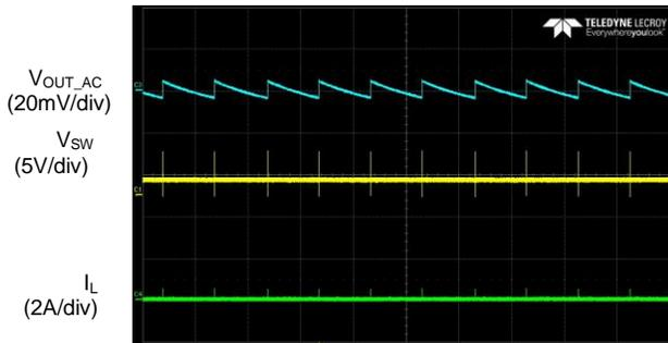
**Output Ripple (I<sub>OUT</sub>=3A)**
