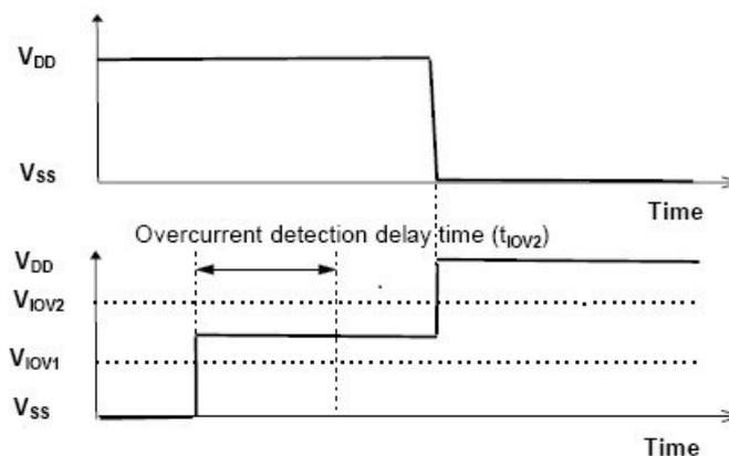
Figure 4. Overcurrent delay time
