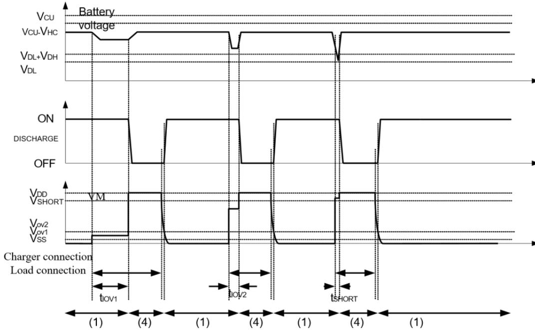
Figure5-2 Overdischarge Current Detection
