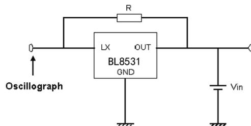
Hold-on voltage test circuit
