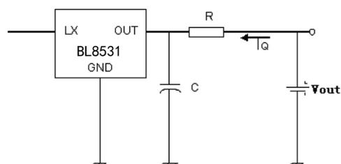
Start-up voltage test circuit
