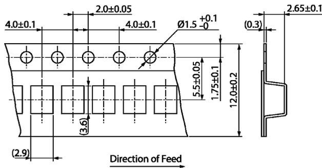
\*Dimension of the Cavity is measured at the bottom side. (in mm)
