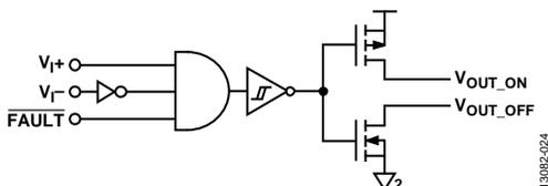
Figure 24. V<sub>I+</sub> and V<sub>I-</sub> Block Diagram
