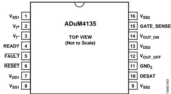
Figure 3. Pin Configuration
