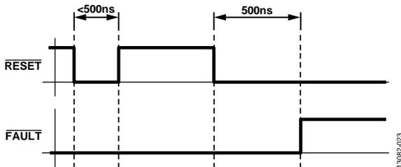
Figure 23. RESET Timing
