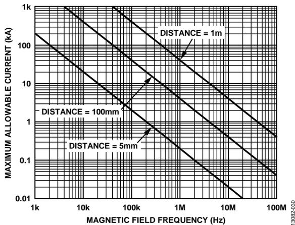
Figure 26. Maximum Allowable Current for Various Current-to-ADuM4135 Spacings
