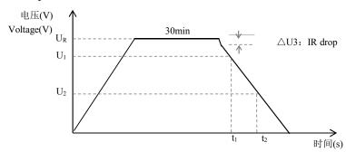
容量计算公式 Capacitance calculation formula:  $C = \frac{I \times (t_2 - t_1)}{U_1 - U_2}$
